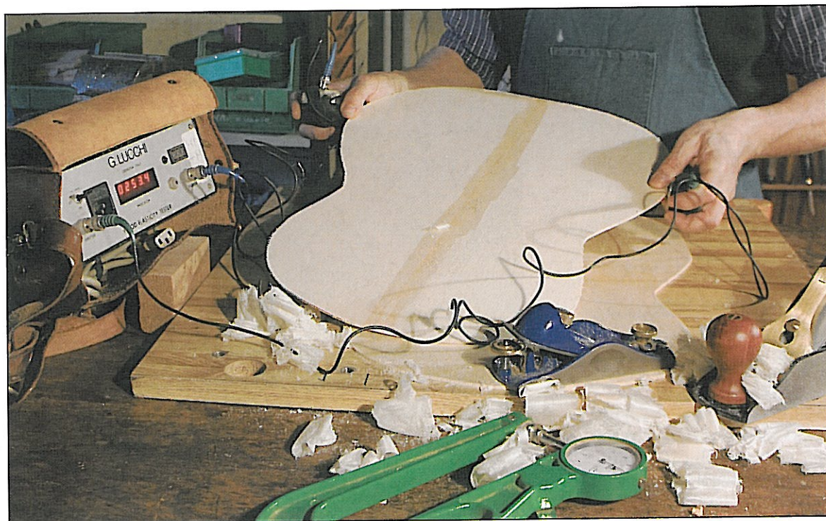
Left: Andrea tests a soundboard using the Lucchi Wood Elasticity Tester, an electronic device that measures the speed of sound in wood. He has been using it since 1984.
