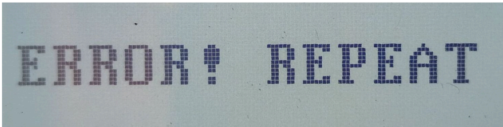
Figure 6.3 — ERROR! REPEAT — instability detected during the SET ZERO procedure
